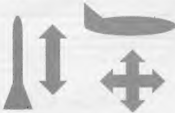
Figure 2-8 Forces acting on a rocket compared to an aeroplane.
