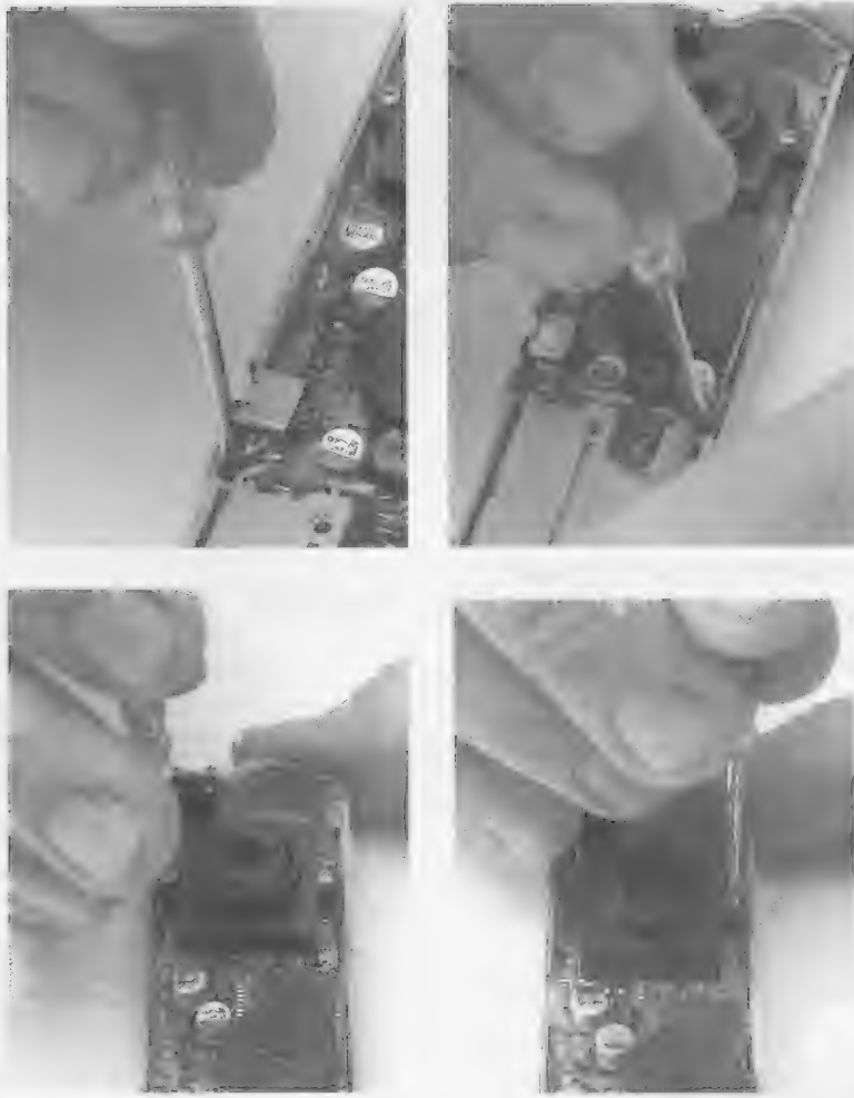
Figure 9-7 Removing the four screws inside the case.
