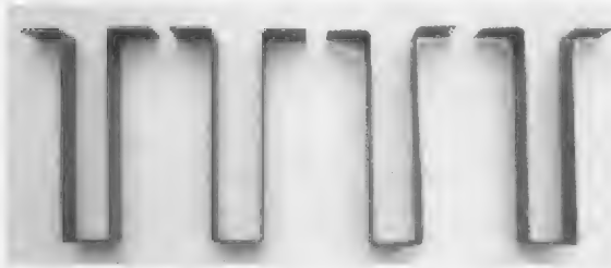
Figure 7-38 Four finished metal brackets.
