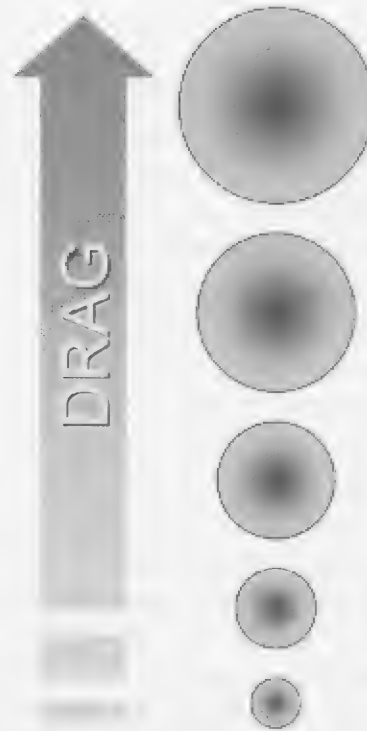
Figure 2-11 How body tube diameter affects drag.
