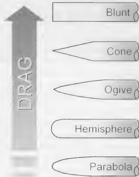
Figure 2-10 How nose cone profile affects drag.
